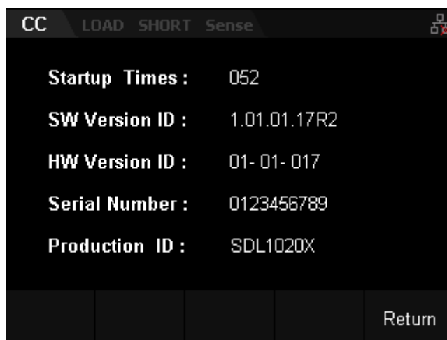
Figure 3-3 System info interface
