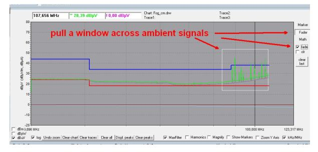
Activate the **Cor** box to see the resulting correction curve.
